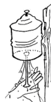
cistern with valve
