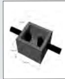
4. Sewerage system junction chamber
